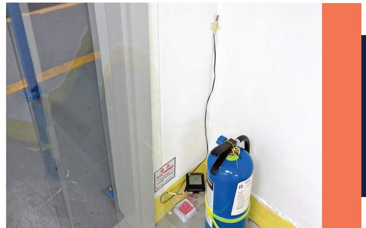
**EL-WIFI-TP logger monitoring warehouse temperature**
