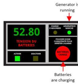
Figure: Generator Starts – Batteries are Charging
