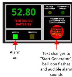
Figure: Battery Charge Drops to 55% or Less
