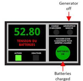
Figure: Batteries are Charged
