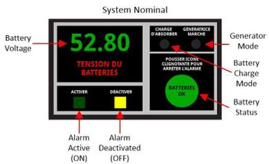
Figure: Typical Meter Display
