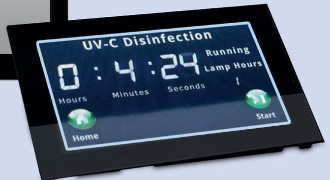
The SGD 70-A is a PanelPilotACE compatible display designed specifically to run projects created in the PanelPilotACE Design Studio. It features a capacitive touch screen and a wealth of hardware interfaces including four 16-bit bipolar analogue inputs, eight digital input/output pins, two alarm outputs, four PWM outputs, RS232 and RS485 comms, CANbus and FTP transfer of logged data via Ethernet.
