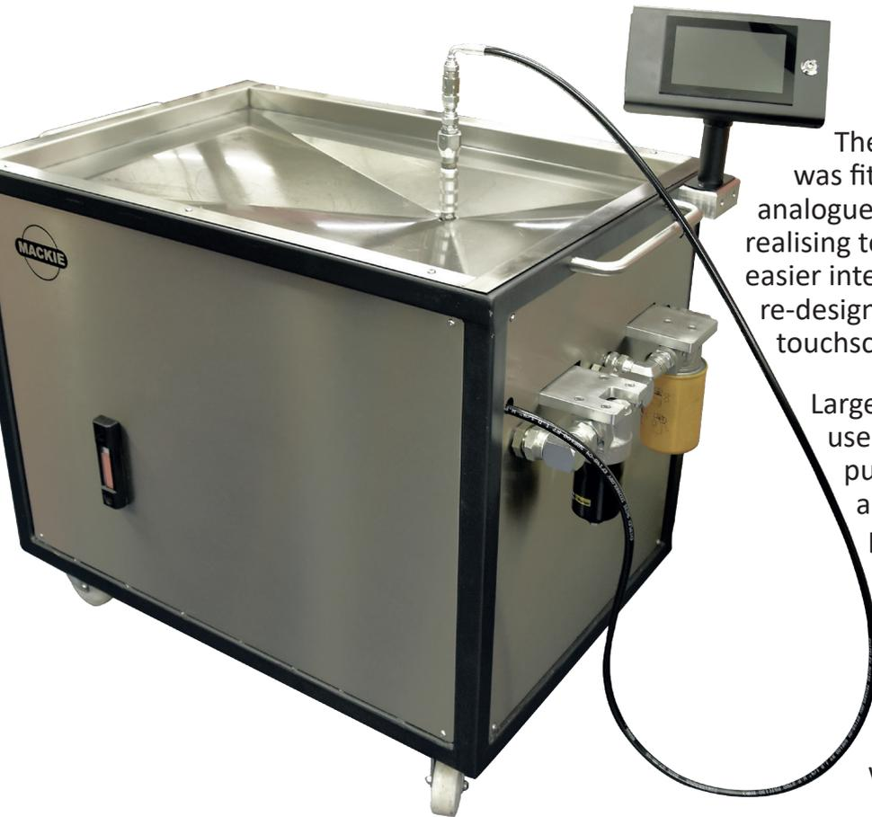
The company's first test machine was fitted with physical buttons and analogue gauges to show these values but realising technicians needed a faster and easier interface, the machine was recently re-designed using Lascar's 7 inch, capacitive, touchscreen display – the SGD 70-A.
