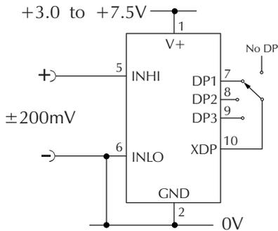
Measuring a single ended input voltage referenced to supply, i.e. the input voltage and the meter's power supply share the same 0V rail. Ensure solder link LCOM is open.
