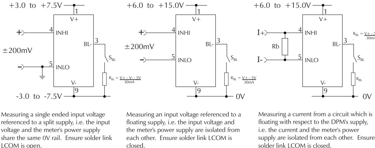
Measuring a single ended input voltage referenced to a split supply, i.e. the input voltage and the meter's power supply share the same 0V rail. Ensure solder link LCOM is open.
