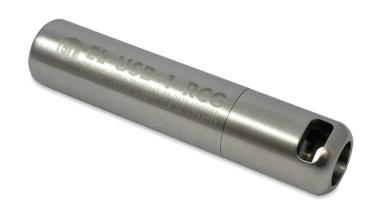
This standalone data logger measures and stores more than 32,000 temperature readings over a -20 to +60°C (-4 to +140°F) range with a resolution of  $0.1^{\circ}$ C ( $0.2^{\circ}$ F).
