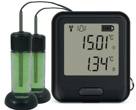
The EL-WiFi-VAC2 measures the temperatures of two probes sunk into glycol bottles, designed to mimic vaccine samples. The probes are connected to the logger via a 160mm Y splitter cable which is provided. Data from the probes is streamed wirelessly over any compatible WiFi network and can be viewed on a PC using free software or on the EasyLog Cloud or App.
