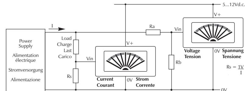
Simultaneous d.c. Voltage and Current Measurement.
