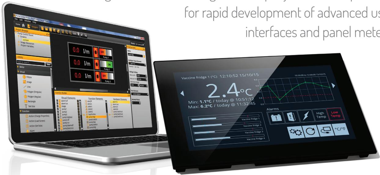
The SGD 70-A is part of the PanelPilotACE range of compatible displays and panel meters. The low-profile display features a 7" capacitive touch screen and a dual-core ARM processor running embedded Linux. The display can be powered from a 5 to 30V d.c. supply and offers users a wealth of hardware interfaces which include four 16bit bi-polar analogue inputs (to a maximum of  $\pm 40V$  d.c.), eight digital input/output pins, two alarm outputs (maximum current sink 10mA) and four 8bit PWM outputs.
