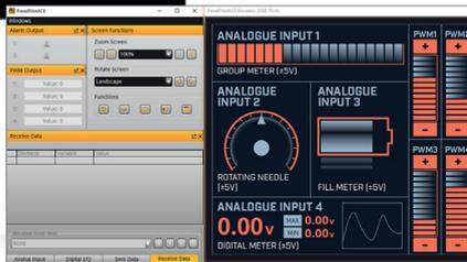
Design Studio's Preview Emulator, which emulates the hardware inputs and outputs, allows students to test their display projects before uploading anything to an actual display.
