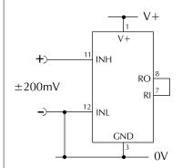
Measuring a single ended input voltage referenced to supply, i.e. the input voltage and the meter's power supply share the same 0V rail.
