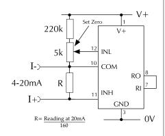
Measuring a 4-20mA loop current. The meter's power supply must be isolated from the 4-20mA current loop.
