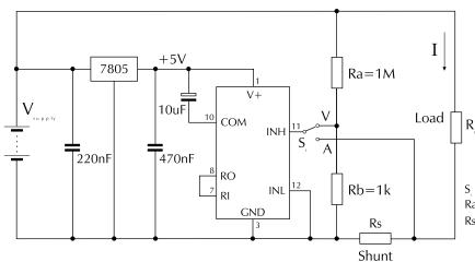
S  $_{\!_{\!\!4}}$  selects between voltage and current display. Ra and Rb shown scaled for 200V  $_{\!_{\!_{\!\!4}588}}$  .
