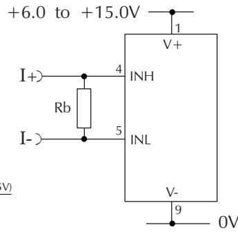
Measuring a current from a circuit which is floating with respect to the DPM's supply, i.e. the current and the meter's power supply are isolated from each other.
