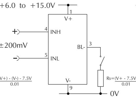
Measuring an input voltage referenced to a floating supply, i.e. the input voltage and the meter's power supply are isolated from each other.
