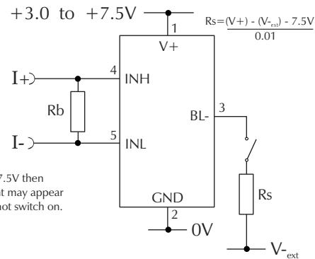
Measuring a current from a circuit which is floating with respect to the DPM's supply, i.e. the current and the meter's power supply are isolated from each other.
