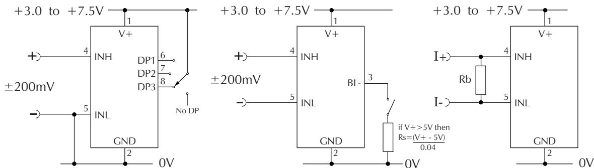
Measuring a single ended input voltage referenced to supply, i.e. the input voltage and the meter's power supply share the same 0V rail.
